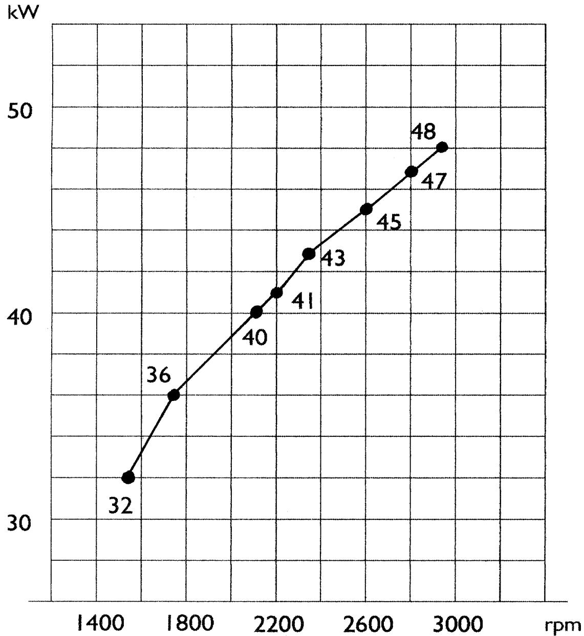
Gross ISO Power 3046 ; Ambient reference conditions : temperature 25°C , relative humidity 30% , pressure 100 kPa (1000 mbar).
