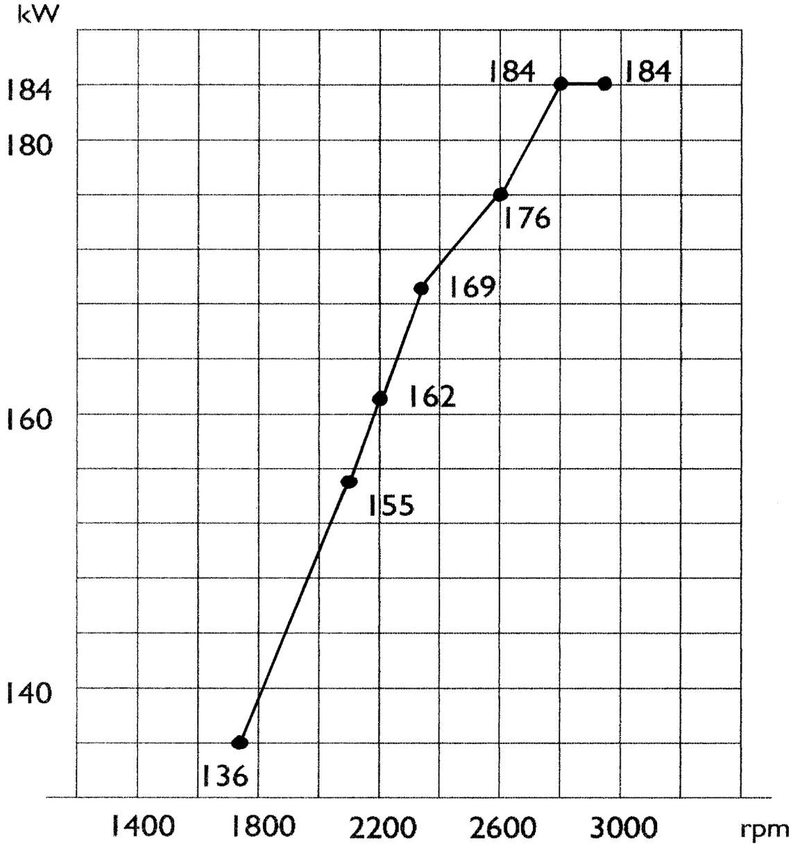
Gross ISO Power 3046 ; Ambient reference conditions : temperature 25°C , relative humidity 30% , pressure 100 kPa (1000 mbar).
